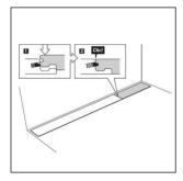
The final plank will need to be cut to length making sure the expansion gap has been allowed for.
