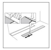
Continue to lay the first row by locking the short ends together, push vertically on the top of the tile or plank and you will hear a click.
