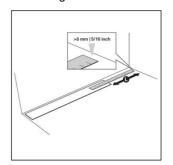
An expansion gap of 8mm is recommended on all sides and up against static objects such as pipes and door frames.
