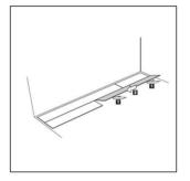
Further planks are positioned into the groove at the same angle and slid to the left to meet the previous plank.
