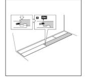
The plank is then lowered and with vertical pressure can be clicked into place.
