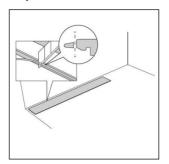
It may be necessary to scribe the first board to the wall, accommodating for an expansion gap
