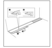
The offcut from the final plank of the first row can be used to begin the next row. Try to avoid cuts of less than 200mm, locate the tongue into the groove of the first row at an angle between 20°-30° and lower to the floor.
